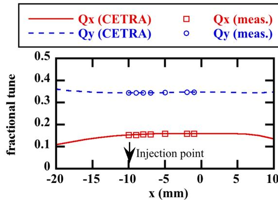
Figure 4: Amplitude dependence of tune.
