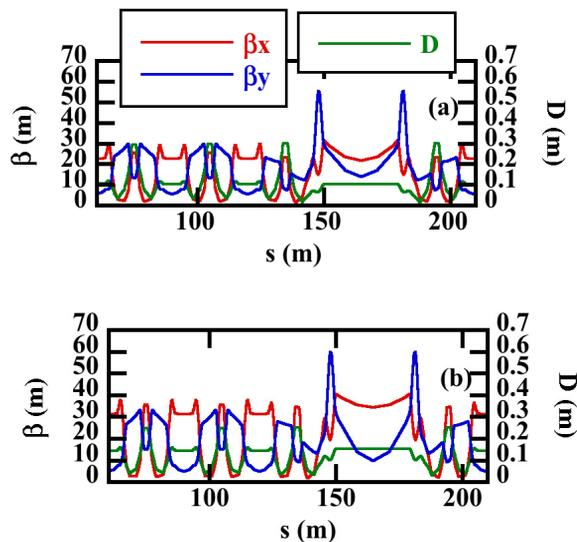
Figure 1: Lattice function of (a) present and (b) new optics.
