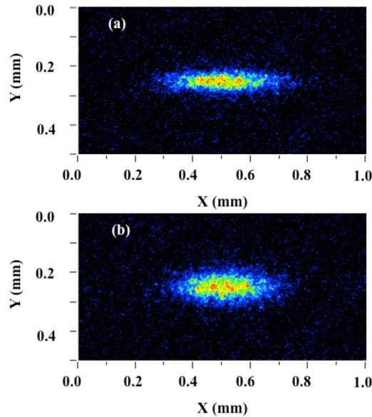
Figure 6: X-ray beam image. (a) Present and (b) new optics.
