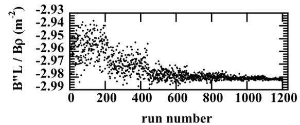
Figure 5: Survey results of a sextupole magnetic field.
