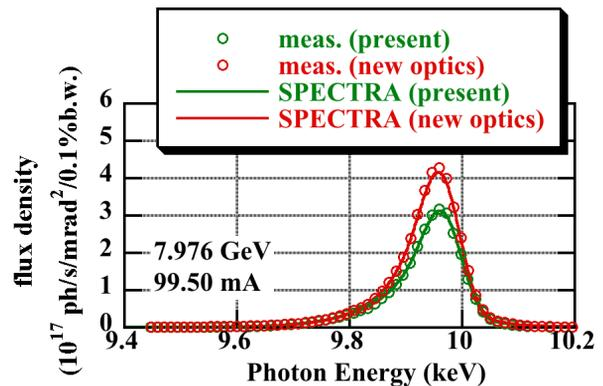
Figure 7: Flux density at the diagnostics beamline II.
