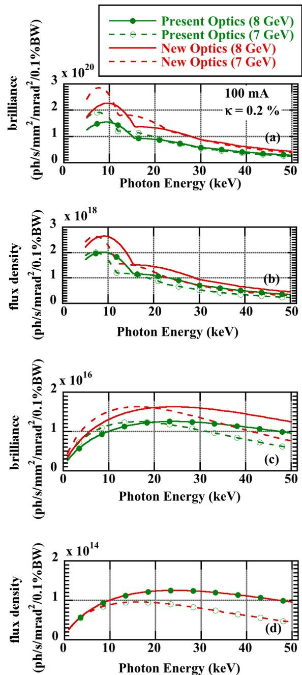
Figure 2: (a) Brilliance and (b) flux density from standard undulator ( $\lambda_u = 32$  mm,  $L = 4.5$  m,  $K_{max} = 2.5$ ). (c) Brilliance and (d) flux density from bending magnet. Calculated by SPECTRA [1].
