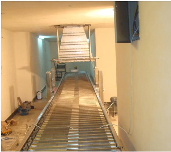
Figure 8: Photo of scan vacuum chamber and transport belt.
