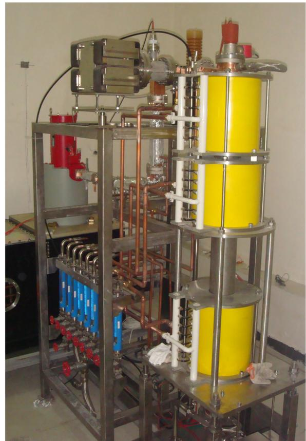
Figure 7: Photo of LINAC of 10 MeV.
