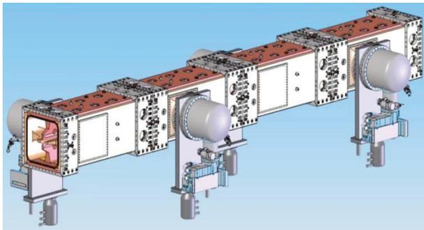
Figure 5: 3-D CAD model of PXIE RFQ.
