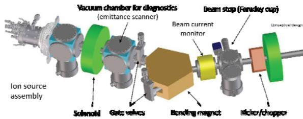
Figure 2: LEBT layout of one arm of 2-solenoid design.
