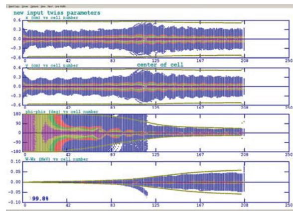
Figure 4: PARMTEQ simulations of the RFQ at 5-mA.
