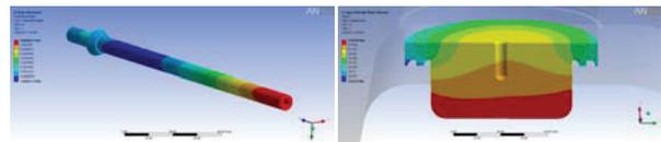
Figure 8: Thermal analysis of  $\pi$ -mode rods (left) indicating that the rod must be water cooled; and slug-tuner (right) does not need to be water cooled.
