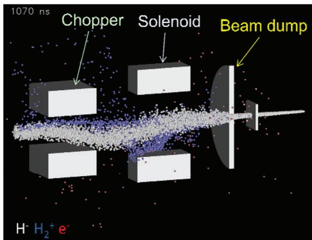
Figure 3: WARP-3D time-dependent simulations of chopper beam dynamics in the LEBT.
