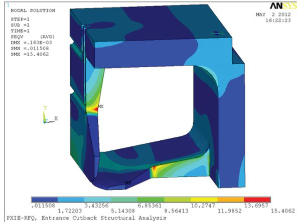
Figure 7: ANSYS Structural analysis of the PXIE RFQ entrance/cutback showing maximum stress of 15.4 MPa, well below the maximum yield stress.
