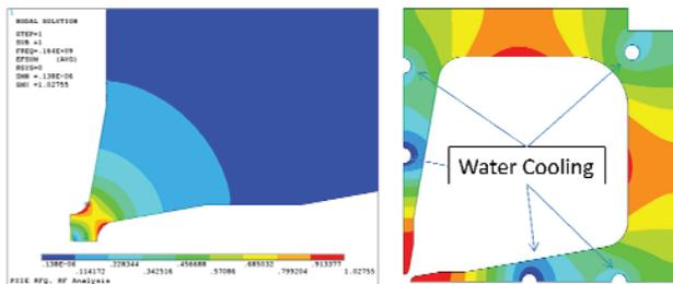
Figure 6: ANSYS simulation studies: RF simulation (left) and thermal simulation (right) with water cooling channel in the vanes.
