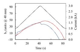
Figure 3: Black: Current cycle. Blue: Measured  $b_3$  component for the search coil configuration with low compensation ratio. Red: Measured  $b_3$  component for the search coil configuration with compensation ratio improved by the voltage divider described in Fig. 1 (right).
