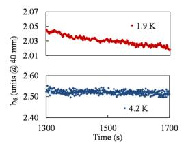
Figure 5: Precision of  $b_6$  measurements during a plateau at nominal current level. Both for operation at 1.9 (red) and 4.2 K (blue).
