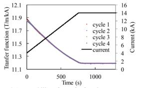
Figure 6: Repeatability of transfer function measurements in four excitation cycles.
