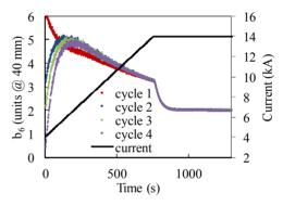
Figure 7: Repeatability of  $b_6$  measurements in four excitation cycles. The multipole depends on the precycling conditions at low field but it is repeatable at nominal field.
