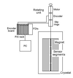
Figure 2: Schematic of the measurement system.
