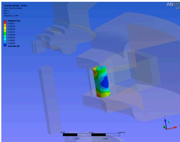
Figure 3: Close-up view showing the field strength in a 0.375" diameter ferrite rod due to the magnetron's axial field.
