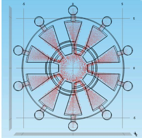
Figure 5: Comsol result showing the fields in the magnetron cavities with ferrite rods.
