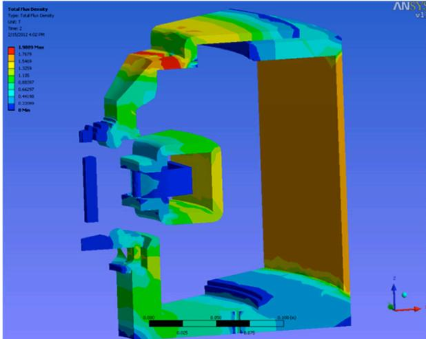
Figure 2: ANSYS model for 36° shows the interaction region, shielding can, control coil pole pieces, and ferrite rod. (The cavity is not part of the magnetostatic model).
