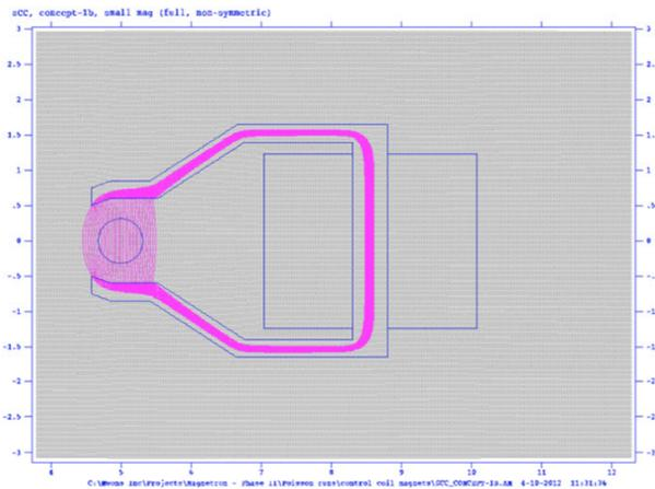
Figure 4: Poisson output graphic showing the control coil pole pieces, control coil region, and the portion of the fields which intersect the ferrite rod.
