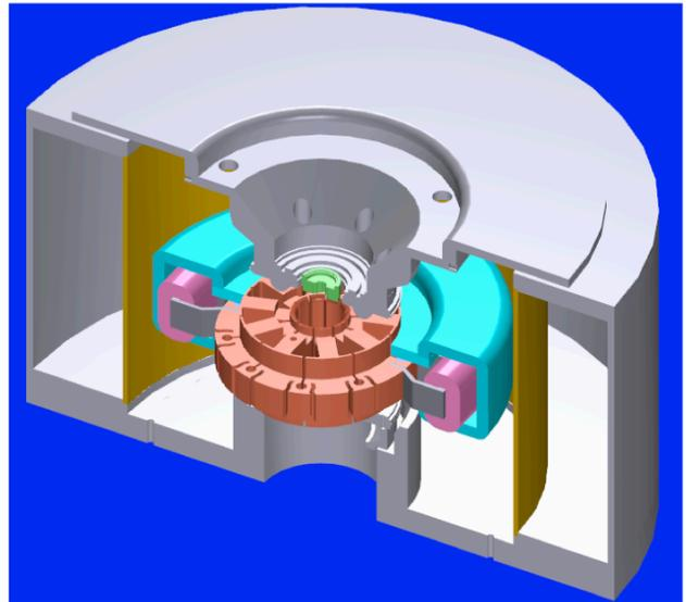
Figure 1: Cutaway view of the magnetron cavity, shielding can, control coils, test solenoid and pole pieces for the low power microwave tests.
