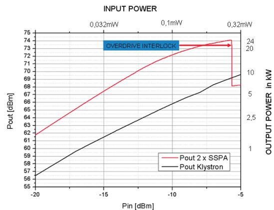
Figure 13: Gain characteristic of the 20 kW SSPA block compared to the klystron used before.
