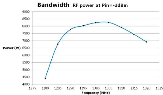
Figure 4: Bandwidth curve of the SSPA.
