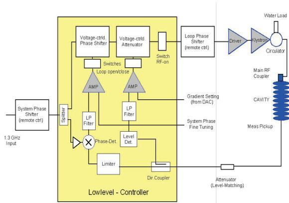
Figure 9: Direct converting (1.3GHz to DC) ELBE low level RF-controller with low-pass filters (LP-Filter) used in the amplitude and phase loop of the LLRF controller.
