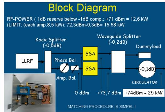
Figure 12: Block diagram of the 20 kW SSPA Block.
