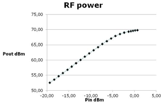
Figure 3: Transfer function of the prototype SSPA.
