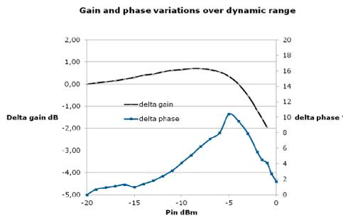
Figure 5: Gain and Phase characteristic of the prototype.
