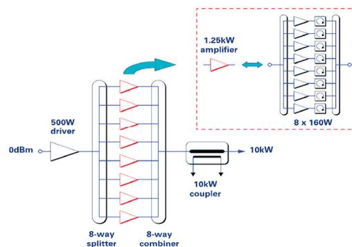
Figure 2: Block diagram of the 8.5 kW SSPA module.
