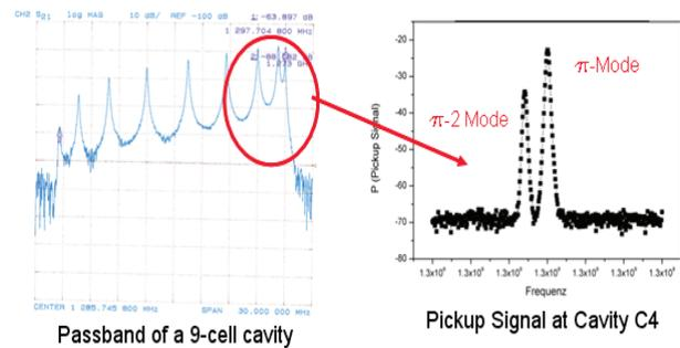
Figure 8: Excitation of the unwanted mode Pi-2 when cavity detuned.
