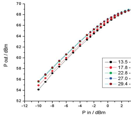
Figure 7: Transfer curve versus temperature of the coolant (Temperature: T=13.5 C to T=29.4 C).
