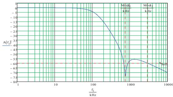
Figure 10: Transfer function of the redesigned low pass filters.
