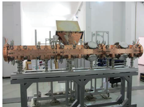
Figure 2: RFQ mounted at the campus of Tsinghua University.
