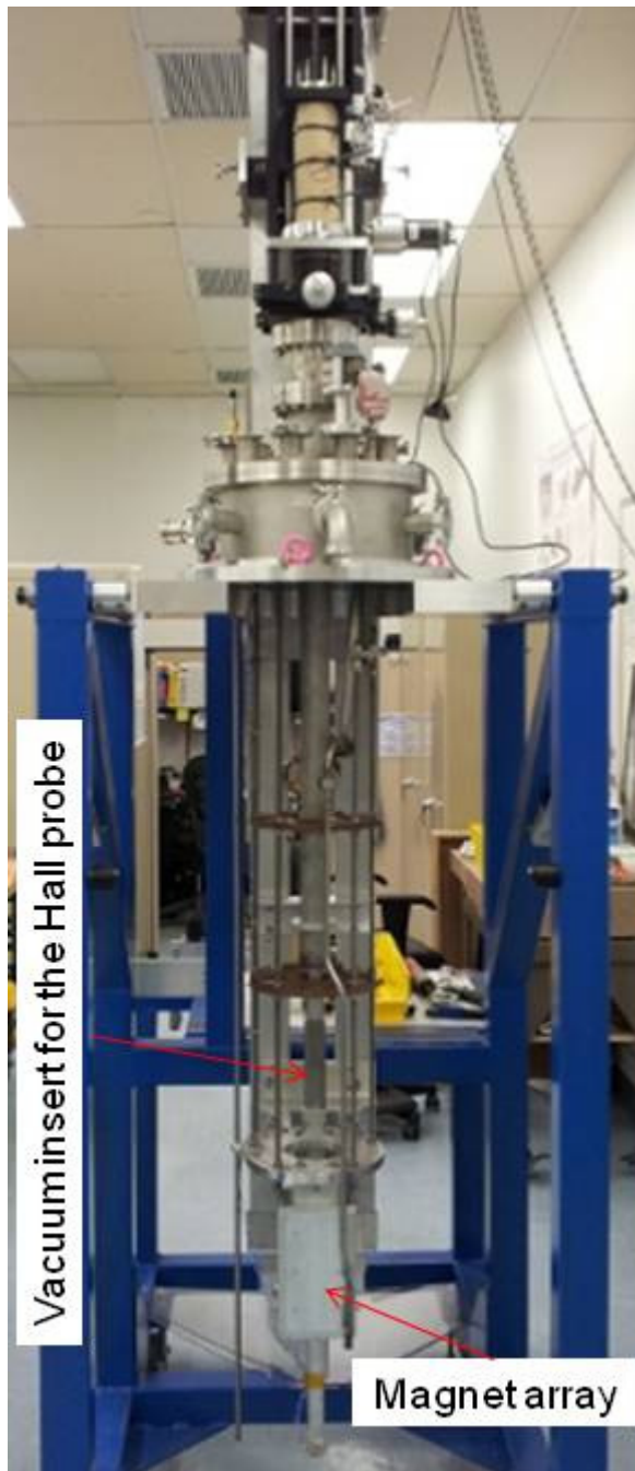
Figure 6: CR47 prototype installed on the VTF.
