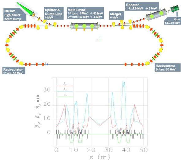
Figure 1: The BERLinPro layout and the Twiss parameters in the ring (beta functions in [m], dispersion in [dm]).
