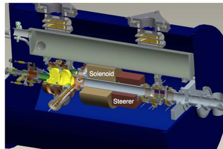
Figure 3: Layout of the SRF injector and SC solenoid.
