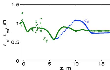
Figure 2: ASTRA simulations of the emittance evolution from the source through the main linac.
