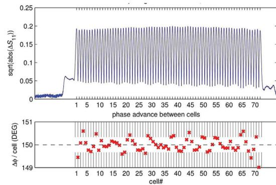
Figure 4: Field flatness and phase advance after tuning.
