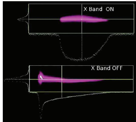
Figure 7: Single bunch charge distribution at the end of the FERMI linac, as measured with an RF deflector: horizontal coordinate corresponds to longitudinal coordinate inside the bunch.
