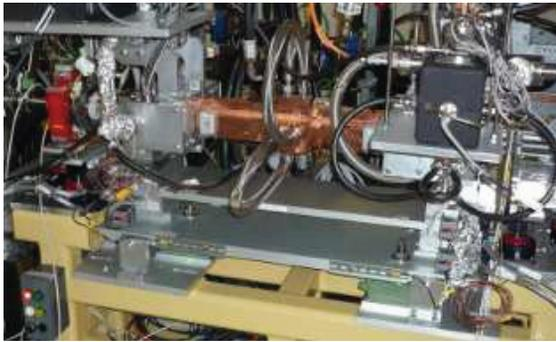
Figure 5: X band structure at the FERMI linac.
