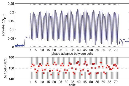
Figure 3: Field flatness and phase advance before tuning at a frequency 1 MHz below the design value.
