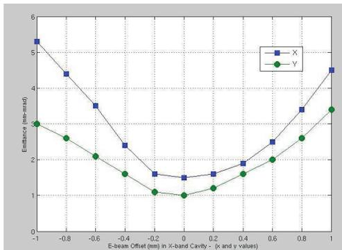
Figure 6: Beam emittance dilution versus offset.
