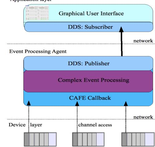
An Event Processing Agent (EPA) aggregates, verifies, analyzes low-level Digital Beam Position Monitor (DBPM) data and distributes summarized results through a Data Distribution Service (DDS) to the GUI. The EPA uses the CAFE API [6, 7], an in-house channel access library, to establish a callback mechanism to the EPICS control system.
