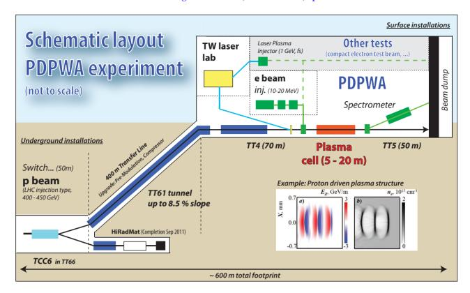
Figure 1: Layout of the experimental installation for a proton-driven plasma acceleration experiment at CERN. The total footprint is about 600 m.
