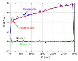
Figure 4: Quadrupole and dipole components after tuning.
