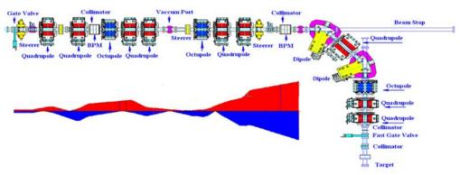
Figure 7: The layout of HEBT.
