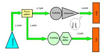
Figure 6: Block diagram of RF transmission subsystem.
