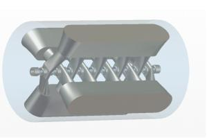
Figure 6: Layout of the first sc CH-cavity.
