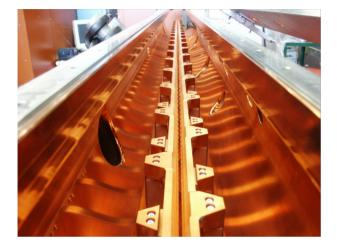
Figure 4: Typical 4-rod-RFQ at 175 MHz.
