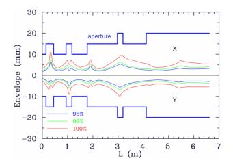
Figure 3: Beam envelopes along the DTL-part of the injector.
