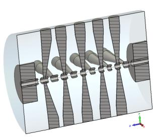
Figure 5: Layout of the first rt CH-cavity.
