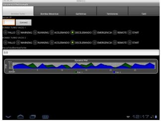
Figure 3: User interface of the Android application.
