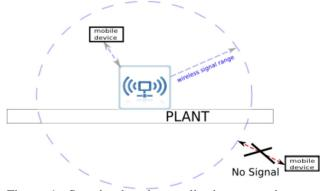
Figure 1: Security based on adjusting transmit-power level.
