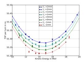
Figure 3: Comparing experimental measurements with simulation results, we observe that for lattices 1, 2 and 3, the agreement in the tof is mostly within 20 ps.
