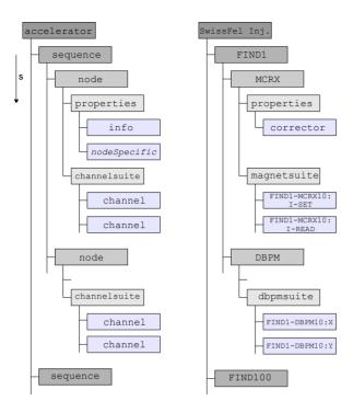
Figure 1: A hierarchical representation of a particle accelerator with associated XML elements (left), accompanied by a partial instance for the SwissFEL Test Injector (right).
