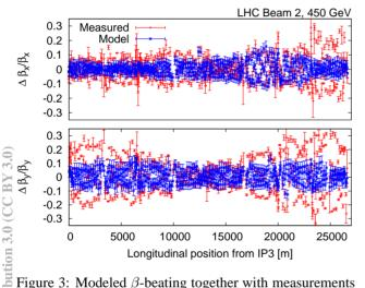
Figure 3: Modeled  $\beta$ -beating together with measurements from the  $19^{th}$  of August 2010 for Beam 2 at 450 GeV.
