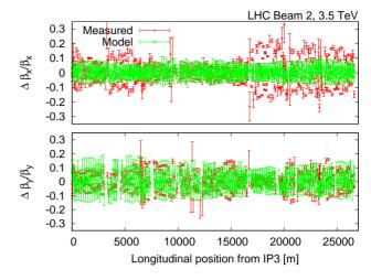
Figure 4: Modeled  $\beta$ -beating together with measurements from the 4<sup>th</sup> of September 2010 for Beam 2 at 3.5 TeV.
