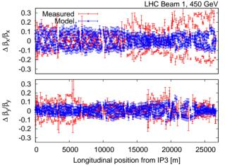
Figure 1: Modeled  $\beta$ -beating together with measurements from the 12<sup>th</sup> of August 2010 for Beam 1 at 450 GeV.
