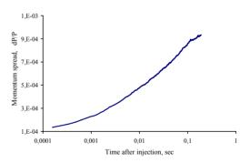
Figure 3: Rms momentum spread of a high intensity Mg beam as a function of time; BETACOOL results.
