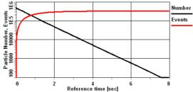
Figure 5: Evolution of the particle number (black) and the integral of ionization events (red) during multiple crossing of 30 keV antiprotons and a Helium jet.
