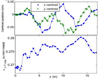
Figure 4: The beam centroid position along the linac (top) and the normalized transverse emittance growth along the linac (bottom) for a proton beam.
