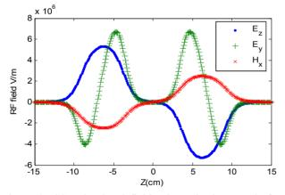
Figure 2: CST simulated fields along the beam axis for  $\beta g=0.08$  and  $\theta=2.5^{\circ}$ . Ey was divided by  $2\theta/\pi$  and Hx by  $-2\theta/(\pi\mu0\beta gc)$ .
