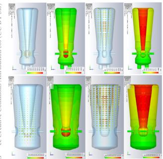
Figure 1: 88MHz QWR  $\beta g=0.08$  (top) & 0.15 CST (bottom) fields. For each cavity, the two left drawings show the electric field in vector and contour representations, while the two right drawings show the magnetic field.
