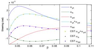
Figure 3: The  $\beta_g$ =0.08 QWR electric and magnetic steering contributions as functions of  $\beta$  for a 1 Joule stored energy at  $\varphi$ =-90°. The curves represent the results of the derived model while the dots were evaluated with CST MWS.
