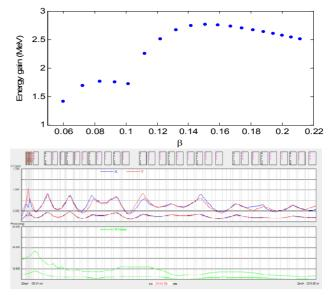
Figure 5: The QWRs energy gain along the linac for a 5 mA deuteron beam (top) and the beam dynamics lattice robustness for a loss of one  $\beta_g=0.08$  QWR (bottom).
