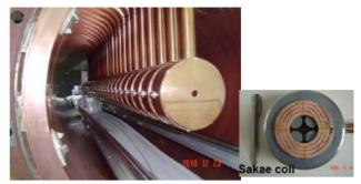
Figure 7: DTL prototype with Sakae coil
