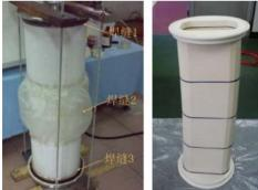
Figure 10: Prototype ceramic chambers for quadrupole (left) and an arc section for dipole (right).
