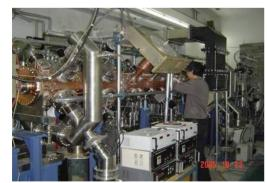
Figure 6: A proton RFQ of 3.5MeV for ADS study has been built at IHEP with 46mA output beam at a transmission rate >93%.
