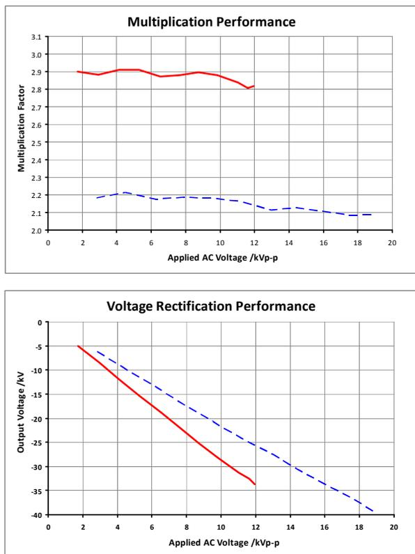
Figure 4: a) Multiplication performance b) Output DC voltage for various Input AC voltages. The solid red line is for 1nF and dashed blue line for 100pF shunt capacitances for a 100MΩ load resistance
