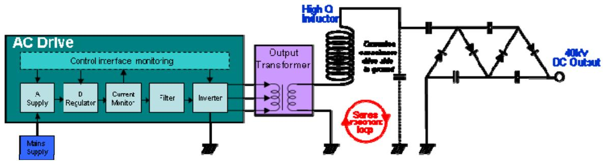
Figure 3: Schematic of the AC drive system, resonant circuit and configuration with the shell structure
