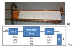
Figure 2: the electrode measurement assembly (a) and the equivalent circuit for simulation model (b).
