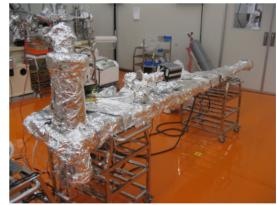
Figure 3: Baking test of chamber R01B1, including a pumping system at 70 L/s, ion gauge and RGA.
