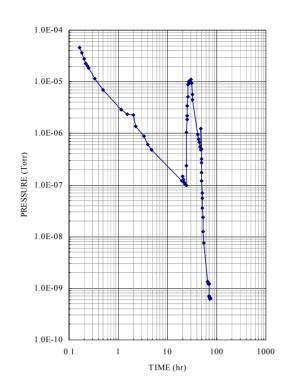
Figure 4: Pumping curve of chamber R01B1 for the baking test. An ultimate pressure  $6.2 \times 10^{-10}$  torr was achieved after the baking test.
