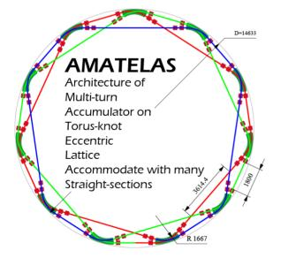
Figure 1: Schematic draw of (11, 3) AMATELAS designed for HiSOR-II.
