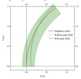
Figure 3: The difference of orbit by field gradient of the bending magnet.
