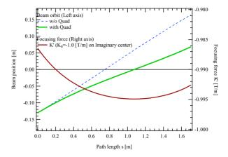
Figure 4: The deviation of focusing force along the orbit in the combined bending magnet.
