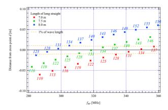
Figure 6: RF frequency and the harmonic number of conditions that the beams collide with each other.
