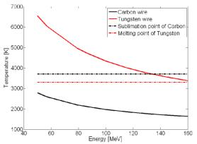
Figure 1: Temperature evolution for 100  $\mu$ m diameter Carbon and Tungsten wire as function of beam energy, for a LINAC4 40 mA, 400  $\mu$ s pulse and typical beam sizes at the monitors locations.
