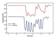
Figure 6: ACEM signal (blue) compared to the LHC-BLM (red) for the CNGS case. The vertical offset is introduced artificially to separate the two curves.
