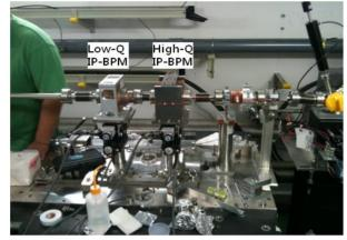
Figure 4: Installed appearance of Low-Q IP-BPM (Left) and High-O IP-BPMs (Right).
