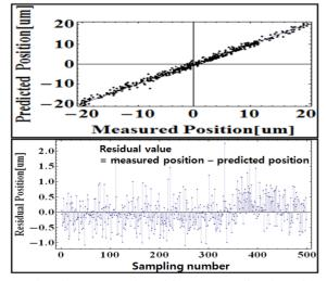
Figure 8: The measured position vs. predicted position (Top). Residual position due to 500 events (Bottom).
