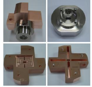
Figure 1: Entire of Low-Q IP-BPM (left up). Reference cavity (right up). Sensor cavity part (left down). Wave guide part (right down).
