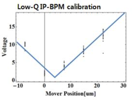
Figure 6: Low-Q IP-BPM calibration run under 40dB amplification condition.
