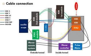
Figure 2: Beam position resolution measurement test scheme for Low-Q IP-BPM.
