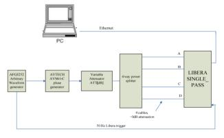
Figure 1: Laboratory test diagram of Libera Brilliance Single Pass
