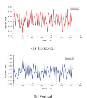
Figure 6: Position results on real beam with mixer added.
