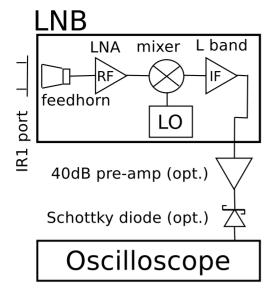
Figure 1: The experimental setup used for the measurement consists of the LNB, amplifier and oscilloscope. It is also possible to rectify the IF signal using a Schottky diode to display the radio frequency (RF) envelope.
