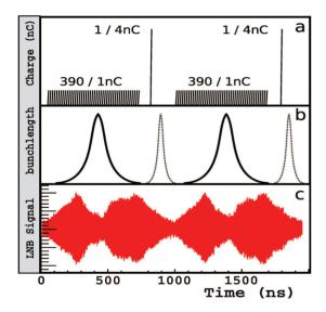
Figure 4: a) Bunch filling pattern of SLS consisting of a train of 390 1 nC bunches with 2 ns spacing and a 4 nC single bunch in the gap. b) bunch length versus bucket number. c) LNB signal of two revolutions at the SLS IR beamline.
