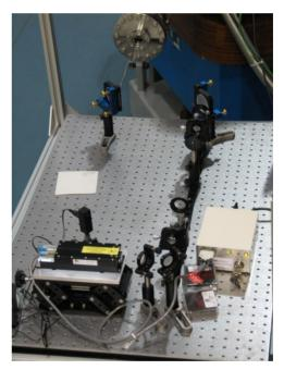
Figure 3: Calibration laser set up with light shaping and steering optics and fast photodiode.
