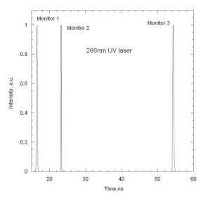
Figure 4: Calibration laser time spectra. Each peak is normalized to its maximum.
