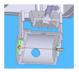
Figure 1: Beam intercepting wire, grounded cylinder and MCP detector assembly on a linear actuator.
