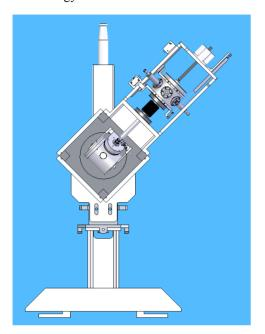
Figure 2: The retractable and adjustable TOF monitor in the beam line.
