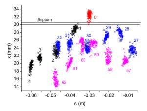
Figure 5: Beam positions at the beginning of the first synchrotron cycle (black "x"), at the end of the first (blue "x") and the second synchrotron cycles (magenta "x"). Numbers near bunches indicate turn number ("0" indicates the injected beam).
