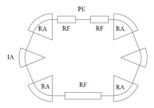
Figure 3: Stacking Ring layout. IA: injection arc; RA: regular arc; RF: rf cavities; PE: positron extraction.
