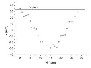
Figure 2: Transverse position of an injected particle at the injection point over 30 successive turns, for an initial momentum deviation  $\Delta p/p_0=+3\,\%$  at a dispersion function  $\eta_{\rm i}=1\,\rm m$ , an initial betatron-oscillation amplitude  $X_{\rm b}=5\,\rm mm$ , a fractional betratron tune  $Q_{\rm x}=0.75$ , and synchrotron damping time  $\tau_{\rm s}=100\mu{\rm s}$  (333 turns).
