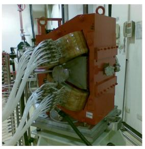
Figure 2: The alpha magnet with vacuum chamber.
