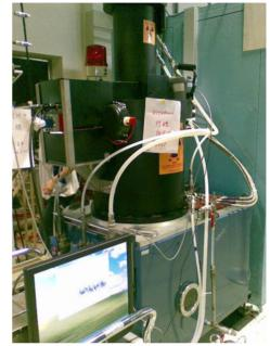
Figure 5: The 35 MW TH2100A klystron system.
