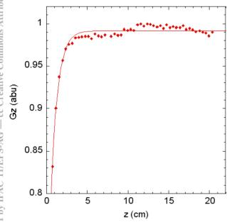
Figure 4: Measured field gradients versus longitudinal position from the mirror plate (i.e. uniformity of gradient along the longitudinal position from the mirror plate).
