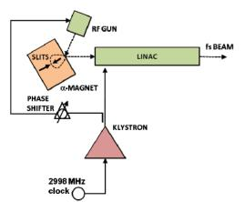
Figure 1: Schematics of the NSRRC low energy thermionic rf gun linac system for ultrashort beam generation with velocity bunching.
