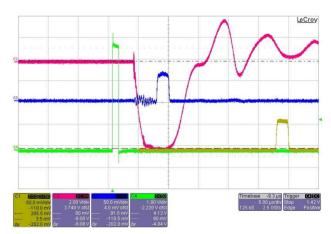
Figure 6: The klystron voltage signal (red) and the klystron output signal at saturation (blue).
