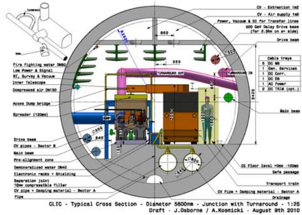
Figure 4: Typical tunnel cross section for CLIC.
