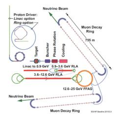
Figure 3: Layout of the Neutrino Factory
