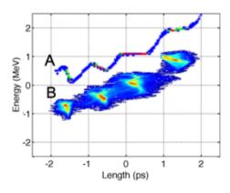
Figure 6: Comparison of measured longitudinal phase space (B) to simulated one (A). (200 pC)
