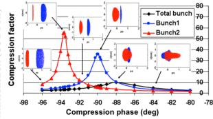
Figure 1: Compression curve for two bunches pulse train at SPARC (simulation, total charge 165pC).
