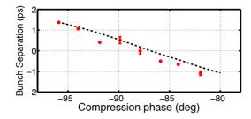
Figure 3: Measured bunch separation for a two bunches train compared to TSTEP simulation (total charge 160 pC).
