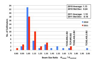
Figure 2: Change in Beam Size Ratio at 450 GeV between 2010 and 2011 B2.
