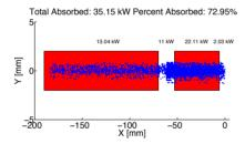
Figure 5: Power distribution on the face of the radiation absorber for the linac-ring design.
