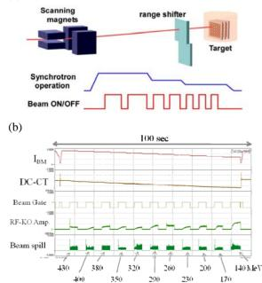
Figure 6: Scheme of the combination scanning (a) and the demonstration of the continuous change of the extracted beam 3606 beam energy (b).
