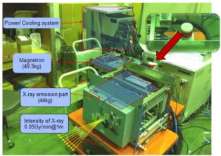
Figure 1: Upgraded X-band 950KeV Linac.
