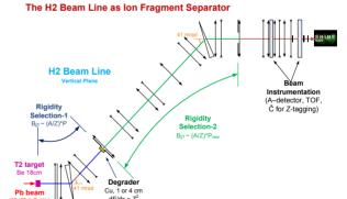
Figure 1: Schematic view of the vertical plane of the H2 beam line, relevant for the ion fragment separation.
