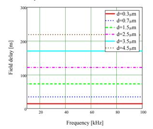
Figure 1: Field delay at peak of field for different titanium coating thicknesses ( $\sigma = 2.5E6$  S/m, a = 31mm) versus frequency.
