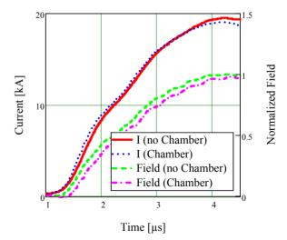
Figure 2: Measured field response of the LHC MKD magnet for 83 kHz sine wave drive current.
