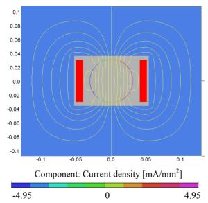
Figure 3: 2D FEM AC simulation model with vector potential lines (yellow) and coloured current density in the chamber coating at 83 kHz, phase of  $90^{\circ}$  and 4.5  $\mu$ m titanium coating.
