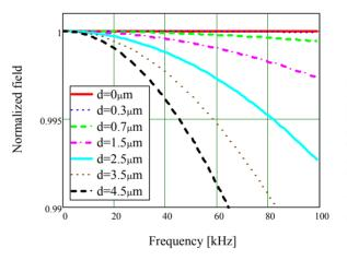
Figure 5: Field attenuation versus frequency for different coating thicknesses.
