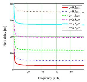
Figure 4: Field delay versus frequency for different titanium coating thicknesses.
