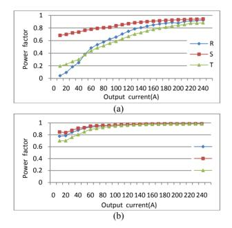
Figure 8: power factor of INVER power supply (a) Normal operation (b) used the shunt APF converter
