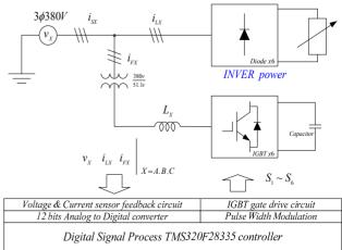
Figure 1: The structure of three-phase shunt APF
