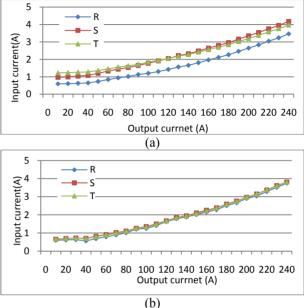
Figure 9: input current of INVER power supply (a) Normal operation (b) used the shunt APF converter
