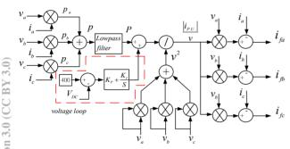
Figure 2: Current and voltage loop compensator block diagram
