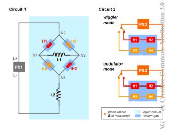
Figure 4: Measurement setup used to test the SCS built to work under conduction cooled conditions.
