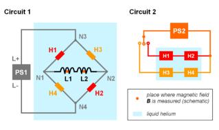
Figure 2: Measurement setup used to test the SCS built to work in liquid helium.
