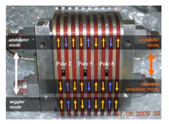
Figure 1: The 9 pole mock-up (COIL) used to demonstrate the feasibility of period length switching in supercoducting insertion devices [5]. The arrows represent the current direction in the winding while the arrow color distinguishes between circuits L1 and L2. Three Hall probes were placed on the poles 2, 5 and 8.
