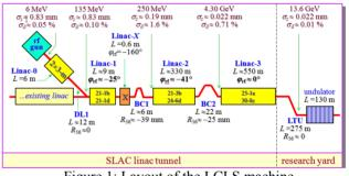
Figure 1: Layout of the LCLS machine.
