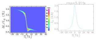
Figure 4: Longitudinal phase space at the undulator entrance with zero R56 at DL2. The L2 RF phase is -33.3° and the heater is 6keV.
