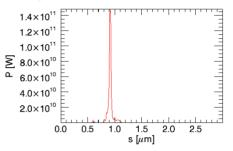
Figure 10: FEL power at the undulator distance of 52.2m with RF phase 17° at L1 and 34.95° at L2.
