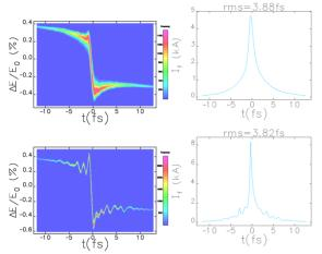
Figure 2: Laser heater effect on longitudinal phase space at undulator entrance with L2 RF phase -33.3°: with laser heater 6keV (top) and without laser heater (bottom). The computation uses 12M particles and 500 bins for longitudinal space charge calculation. DL2  $R_{56} = 0.133$ mm.
