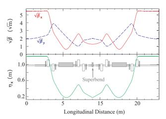
Figure 2: Optical functions of the storage ring.
