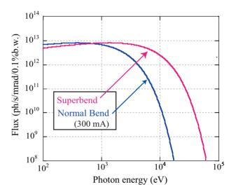
Figure 3: Spectra of photon Flux from the bending magnets.
