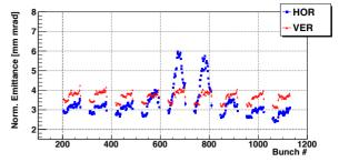
Figure 2: Bunch by bunch emittance snapshot at flat top.
