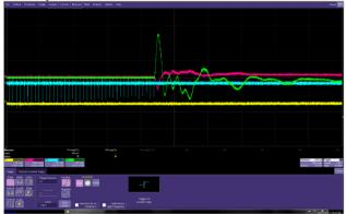
Figure 8: Scope display: first injection kicker (yellow), both extraction kickers (magenta and green) and the BPM signal from successive passes of the beam (cyan).
