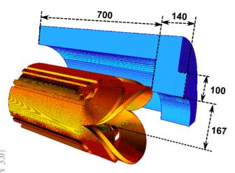
Figure 4: A design for the F magnet, showing half the magnet with dimensions in mm. Coils and an iron yoke are shown.
