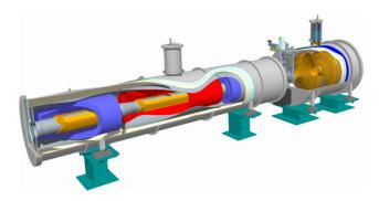
Figure 3: Conceptual engineering of magnet module and RF cavity straight.
