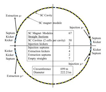
Figure 1: Layout of the FFAG ring.
