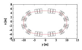
Figure 5: Layout of the advanced FFAG based on the arcs with different radii ("the egg-shaped ring").
