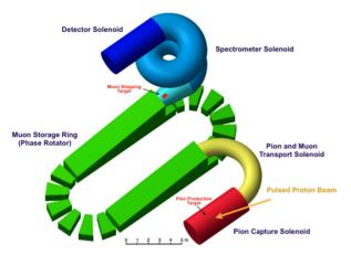
Figure 1: Conceptual layout of the PRISM/PRIME.
